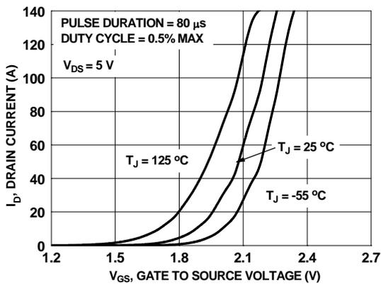
Figure 5. Transfer Characteristics
