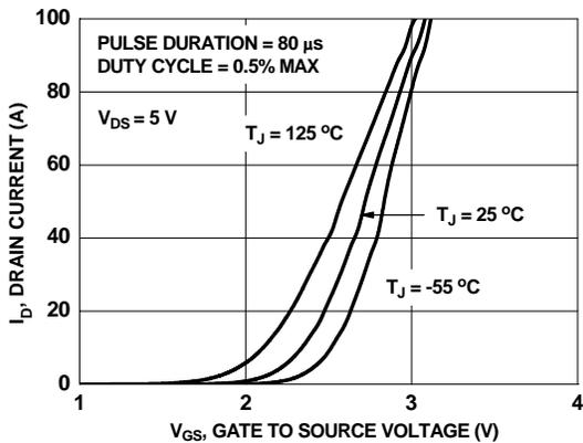
**Figure 5. Transfer Characteristics**
