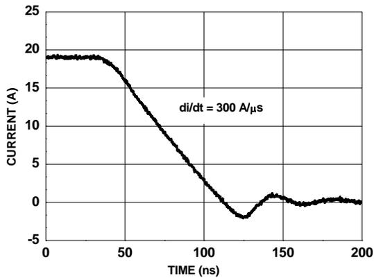
Figure 14. FDMS8026S SyncFET body diode reverse recovery characteristic
