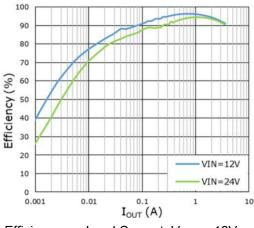
3. Efficiency vs. Load Current, VOUT = 12V
