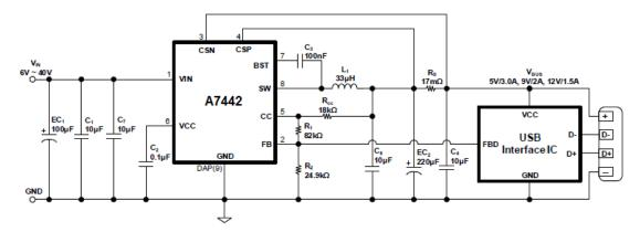
Typical Application Circuit for High Current Output
