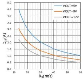
Figure 1. Constant Current Limit vs. Sensing Resistor
