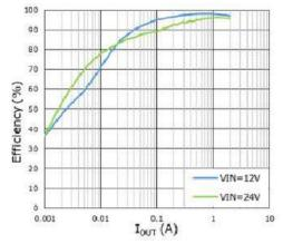
4. Efficiency vs. Input Voltage
