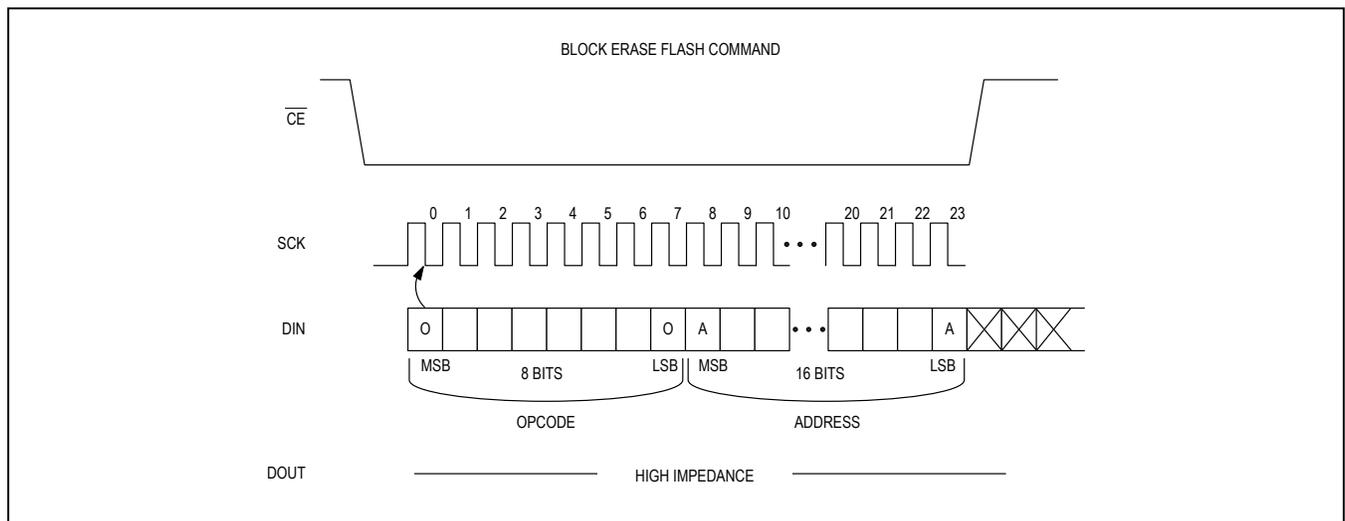
Figure 20. Block Erase Flash Opcode Command Protocol
