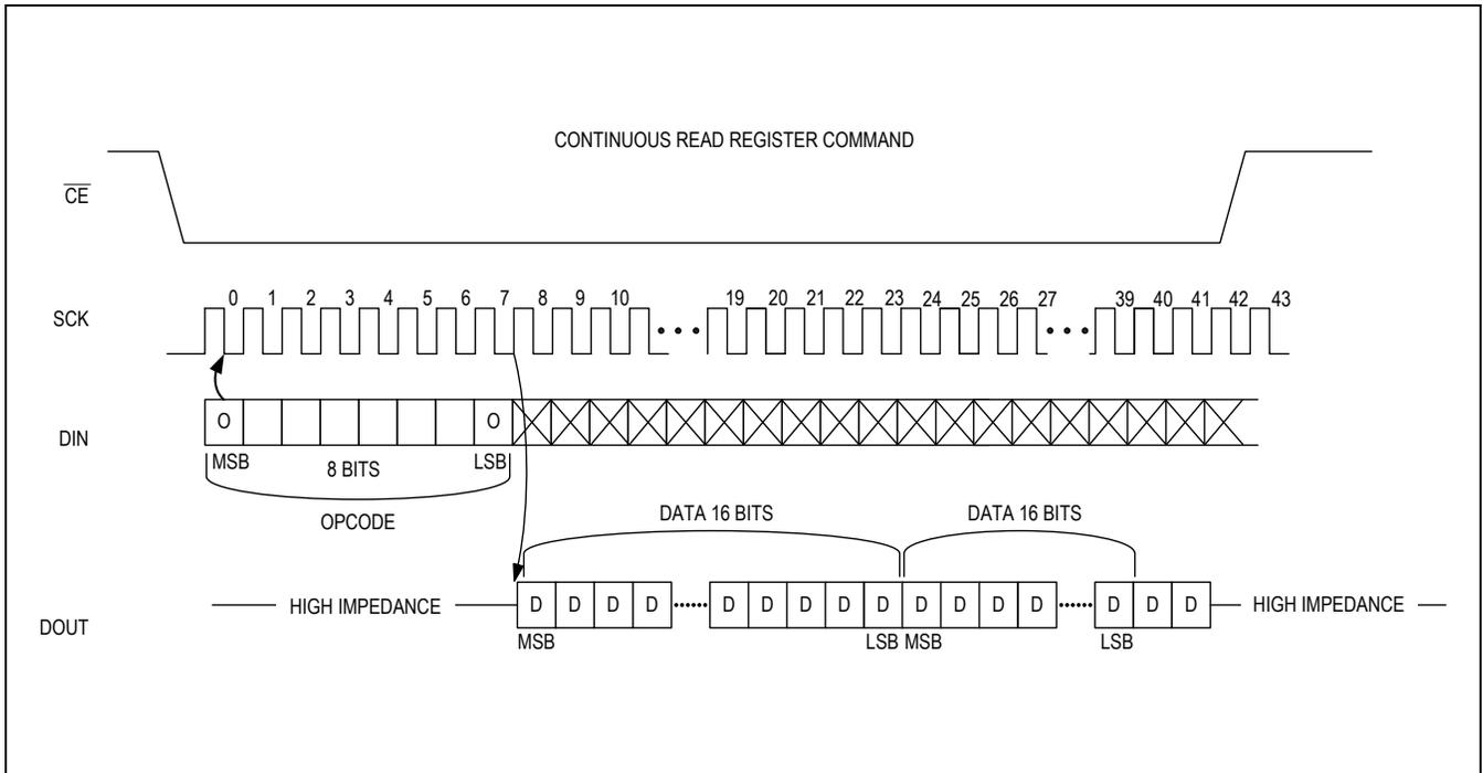
Figure 15. Continuous Read Register Opcode Command Protocol
