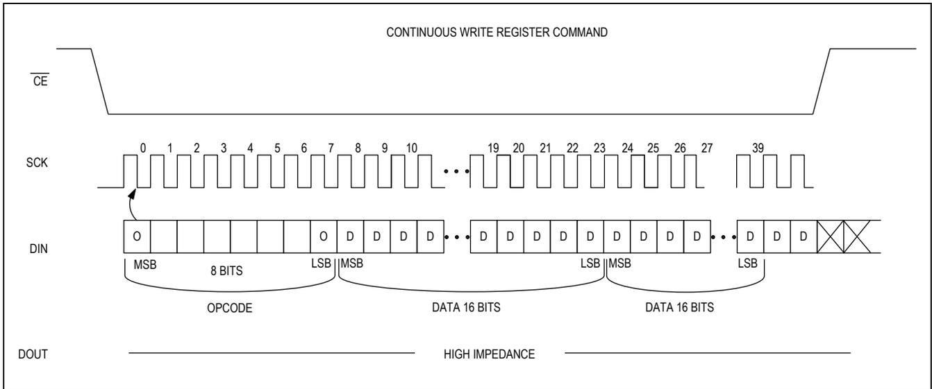
Figure 17. Continuous Write Register Opcode Command Protocol
