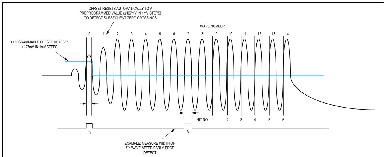
Figure 5. Early Edge Detect Received Wave Example
