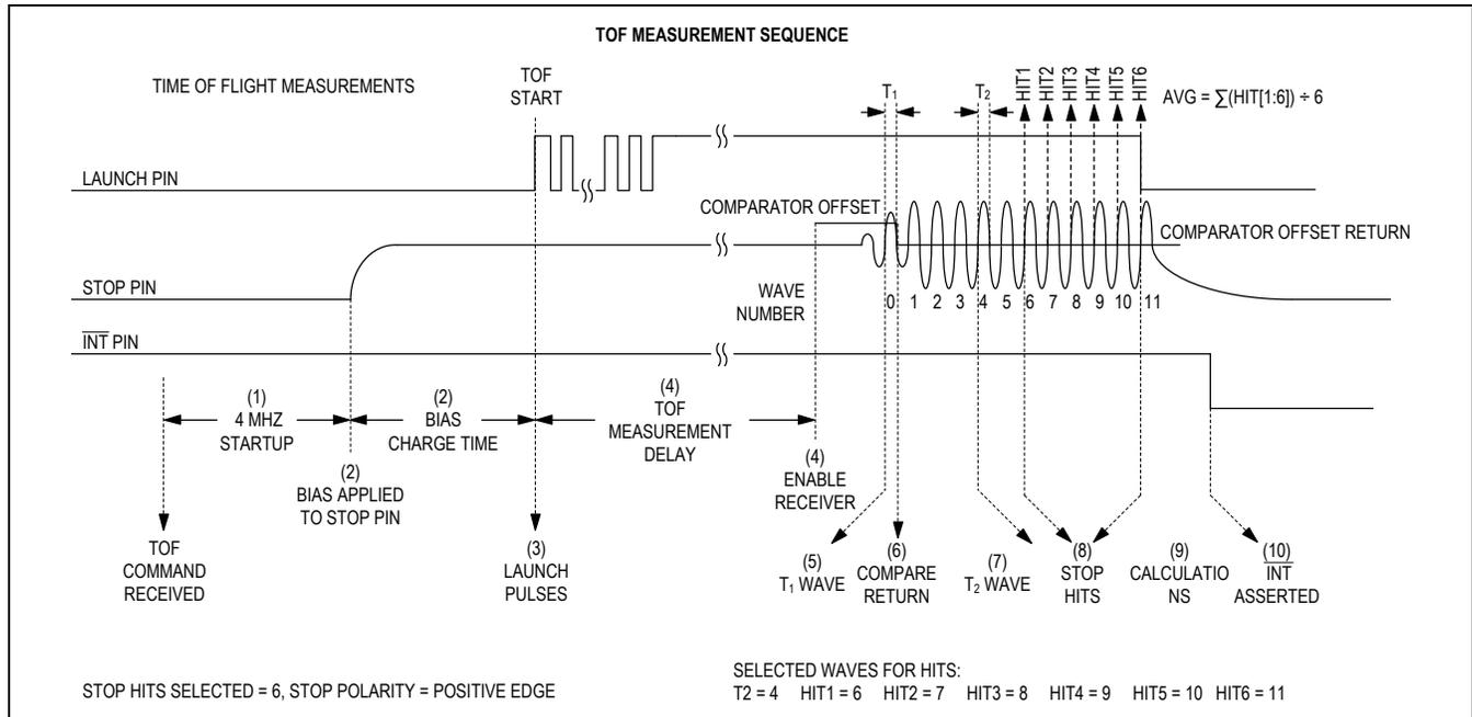
Figure 3. Time-of-Flight Sequence
