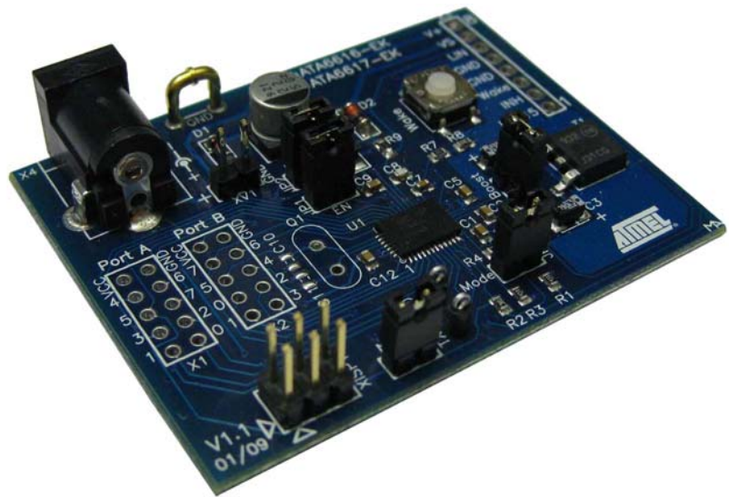
Figure 1. Atmel ATA6616-EK/ATA6617-EK Development Board
