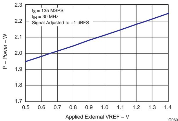
Figure 65. Total Power Consumption versus External VREF
