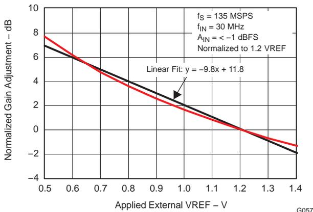
Figure 62. Signal Gain Adjustment versus External Reference (VREF)
