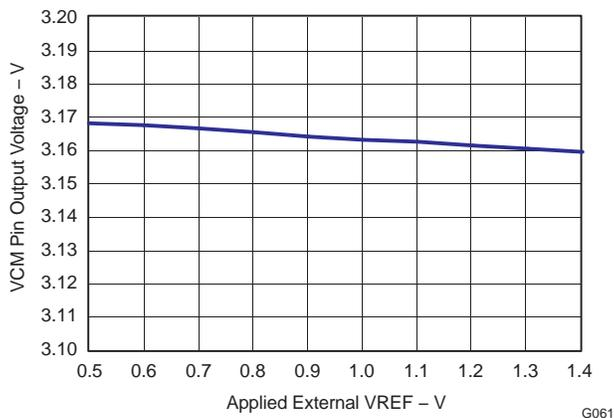
Figure 66. VCM Pin Output versus External VREF
