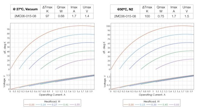
**Note**: Performance data is specified for optimal optimal conditions (TEC hot side is stabilized at ambient temperature). Heatsink thermal resistance is not included into estimations. Use TECCad Software for estimations under different conditions.
