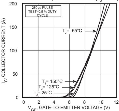
FIGURE 6. Transfer Characteristics
