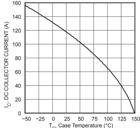
FIGURE 9. DC Collector Current vs Case Temperature
