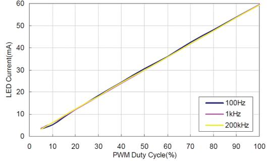
Fig.5 LED Current VS PWM Dimming (3S3P LEDs)
