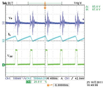
Fig.9 Switching Waveform(10S1P)
