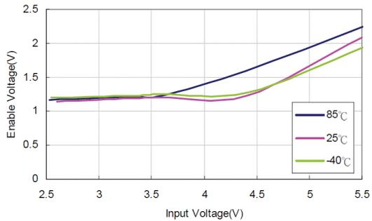
Fig.8 Enable Voltage VS Input Voltage
