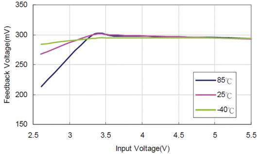
Fig.7 Feedback Voltage VS Input Voltage
