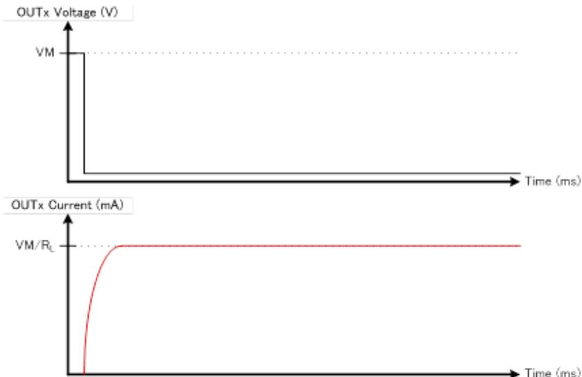
**Case 2: Timer enable bit (C8) is 1 and Energizing Timing bits (C4:C1) are 0000**
