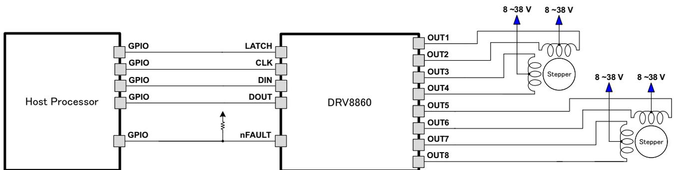
Example Configuration 3: DRV8860 Drives Two Unipolar Stepper Motors
