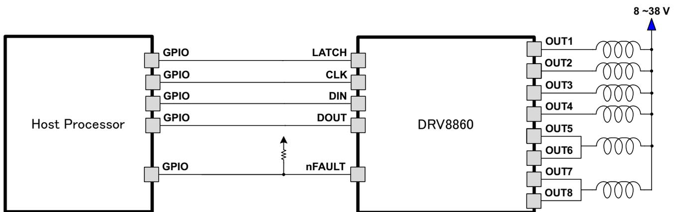
Example Configuration 2: DRV8860 Drives Multiple Low Side Loads With Parallel Configuration
