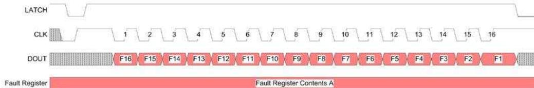
Reading Fault Register – Daisy-Chain
