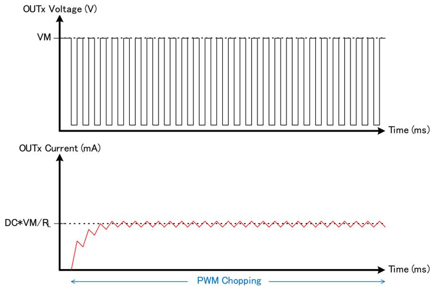
**Case 3: Timer enable bit (C8) is 1, Energizing Timing bits (C4:C1) are NOT 0000, and PWM Duty bits (C7:C5) are NOT 000**
