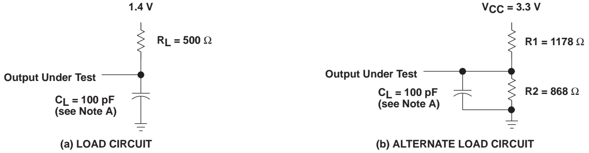
Figure 3. Low-Voltage Load Circuits for Timing Parameters
