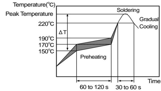
[Allowable Reflow Soldering Temperature and Time]
