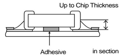
[Standard Conditions for Flow Soldering]
