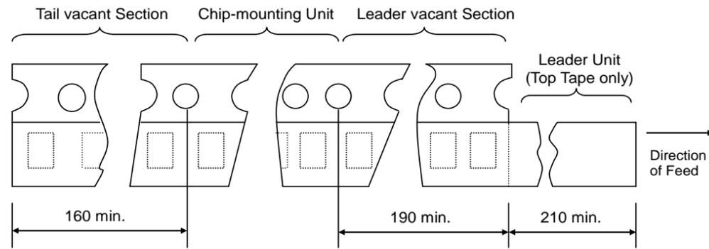
5. Accumulate tolerance of sprocket holes pitch = +/-0.3mm/10 pitch
