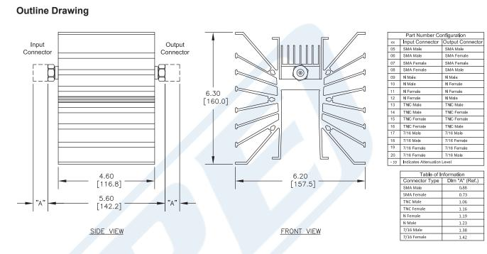
30 dB Fixed Attenuator, SMA Male To SMA Female Directional Black Aluminum Heatsink Body Rated To 300 Watts Up To 3 GHz from Pasternack Enterprises has same day shipment for domestic and International orders. Our RF, microwave and millimeter wave products maintain a 99% availability and are part of the broadest selection in the industry.
