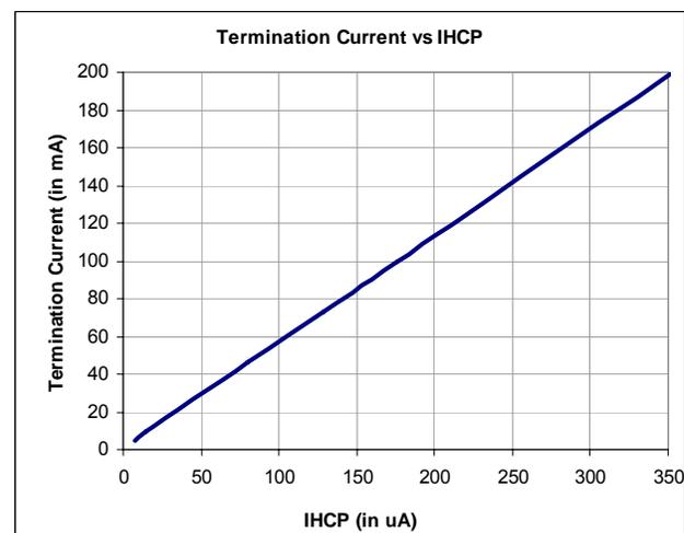
The termination current is always roughly 10% of the maximum charge current set by the HCP resistor R<sub>HCP</sub>.
