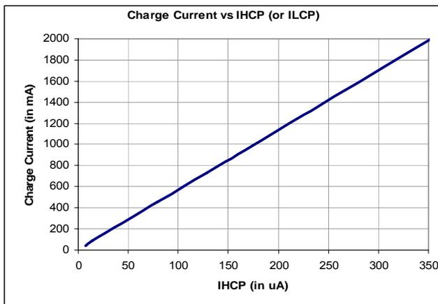
Using the table above it can be seen that for a programming current value of 175μA, the corresponding maximum charge current is 1A.
