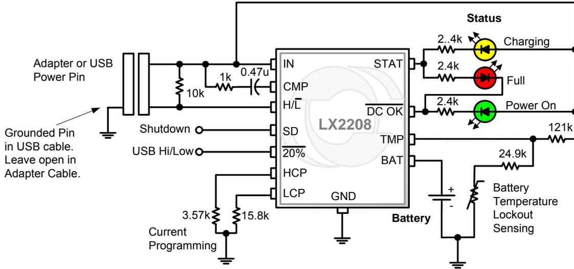
**Figure 1** – Typical Application – 2A adapter charge current and 500mA or 100mA maximum USB charge currents. A grounded spare pin in the USB power cable can be used to sense when the 500mA USB current power source is being used. This application also uses three LED indicators for Power attached, Battery Charging and Battery Full. This configuration also implements circuitry to lockout battery charging if the battery is less than 0°C or greater than 60°C.
