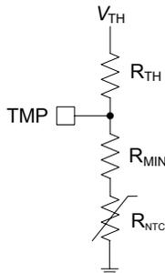
Using a value of  $R_{MIN}$  that is equal to the thermistor temperature at 60°C works well; therefore, for this example, set the value of  $R_{MIN}$  to 24.9k. This has the effect of adding 24.9k to the thermistor resistance values so it becomes 352kΩ at 0°C, 125kΩ at 25°C and 49.8kΩ at 60°C.
