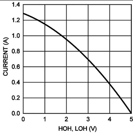
Figure 2. Peak Source Current vs Output Voltage
