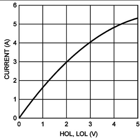
Figure 3. Peak Sink Current vs Output Voltage
