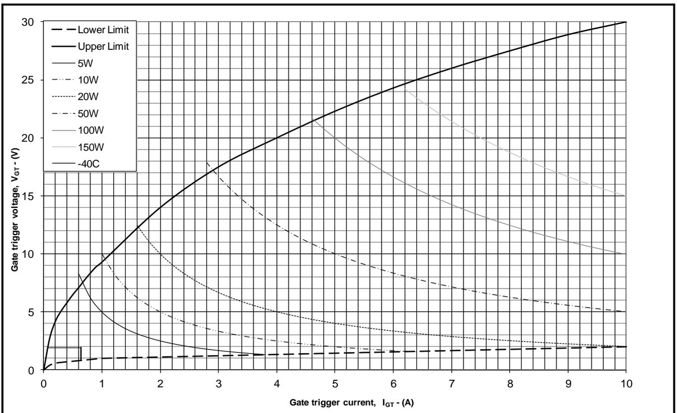
Fig. 15 Gate characteristics
