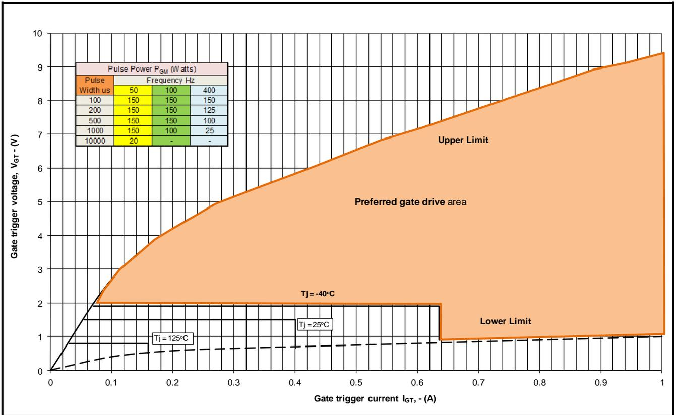
Fig14 Gate Characteristics
