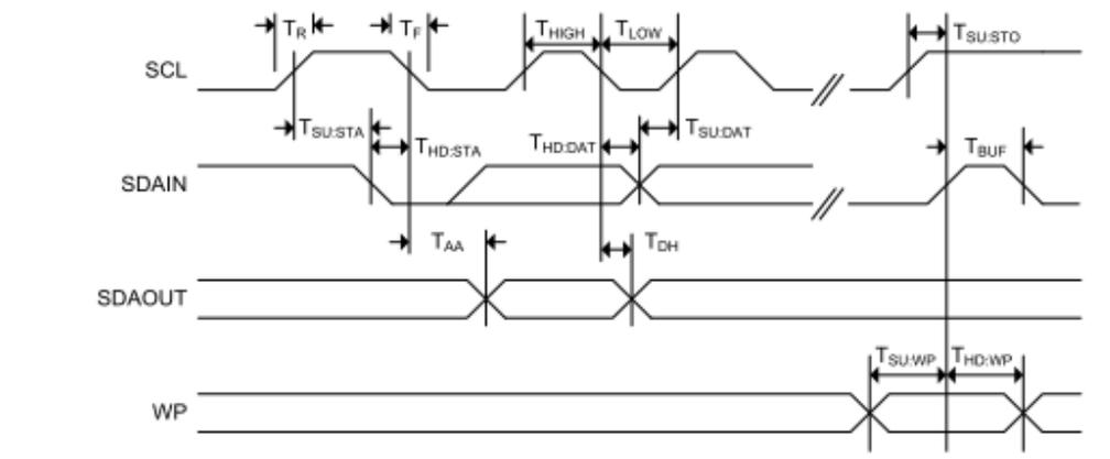
Figure 12. Write Cycle Timing
