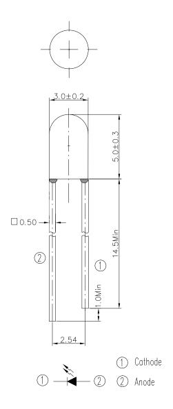
Note: Tolerances unless dimensions ±0.25mm
