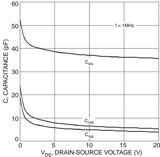
Fig. 9 Typical Capacitance
