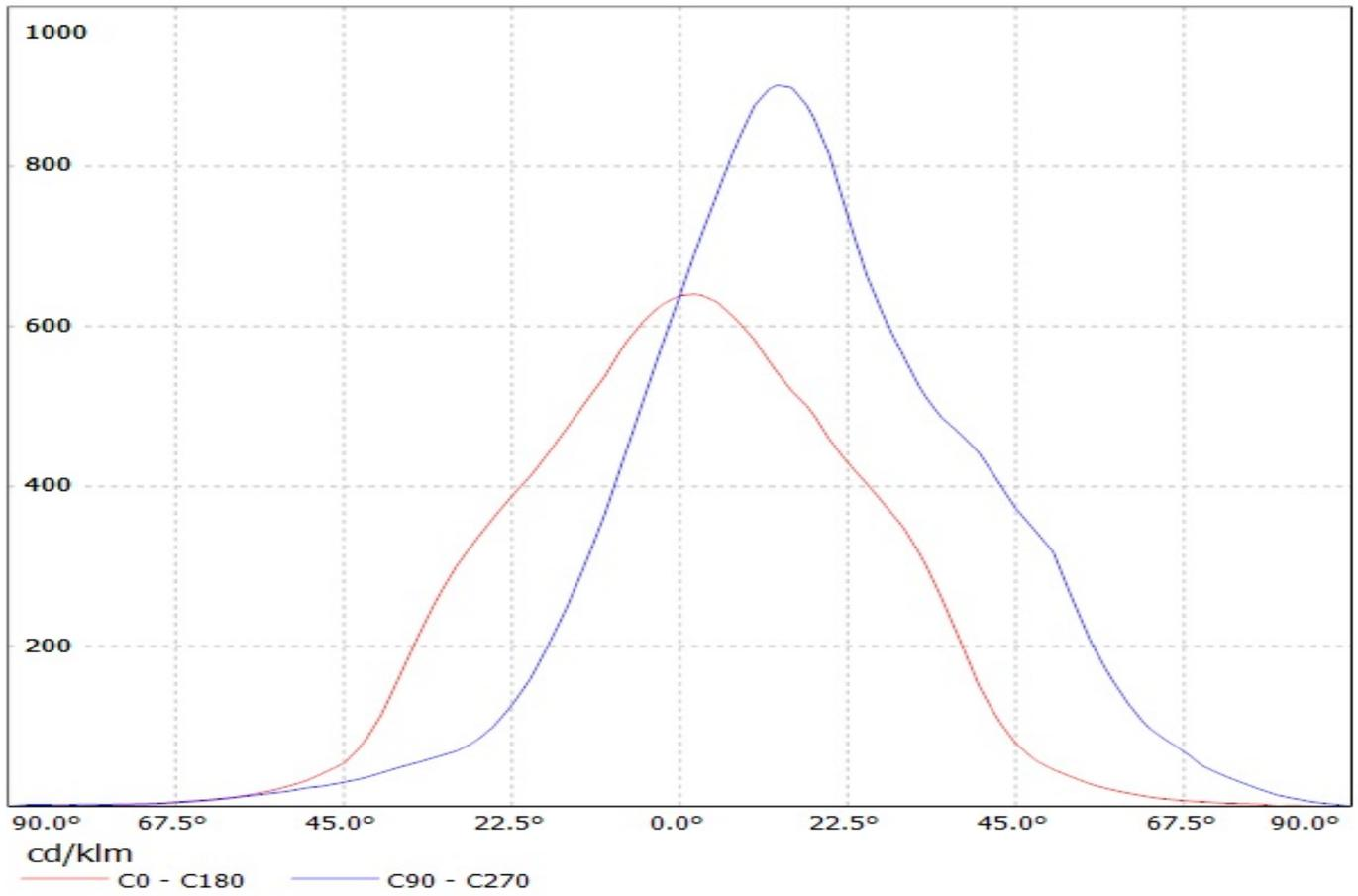
Luminaire: Ledil Oy CN13169\_LENA-WAS-DL (Cree CXA20 698lm @ 250mA) Efficiency=75%
