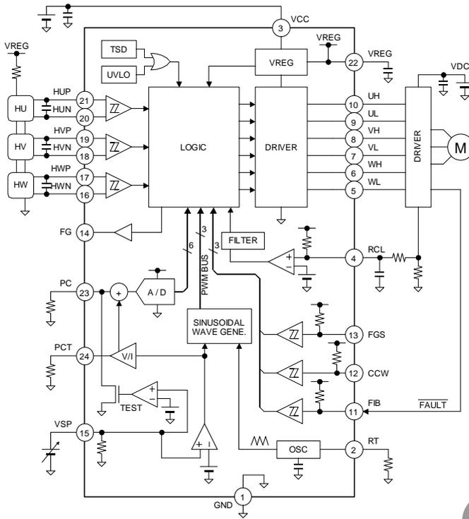
Figure 2. Block diagram
