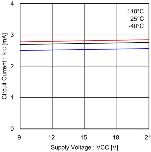
Figure 9. Circuit current
