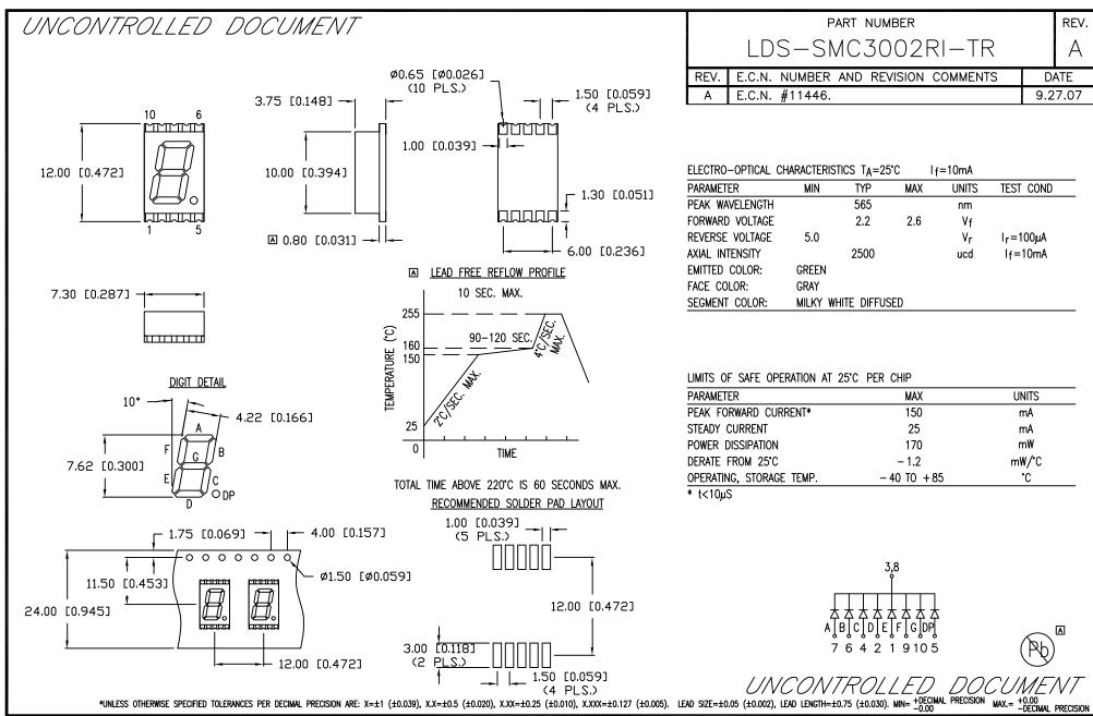
0.30" SMT 7 SEGMENT DISPLAY, COMMON CATHODE, 565nm GREEN LEDS, GRAY FACE WITH WHITE SEGMENTS.
