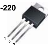
1.Gate 2. Drain 3. Source
