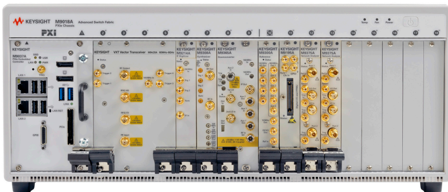
M9420A VXT PXIe vector transceiver placed inside the M9018A PXIe chassis
