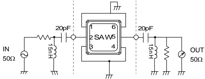
Fig.1 Measuring circuit
