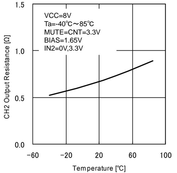
Figure 13. CH2 Output ON resistance characteristic
