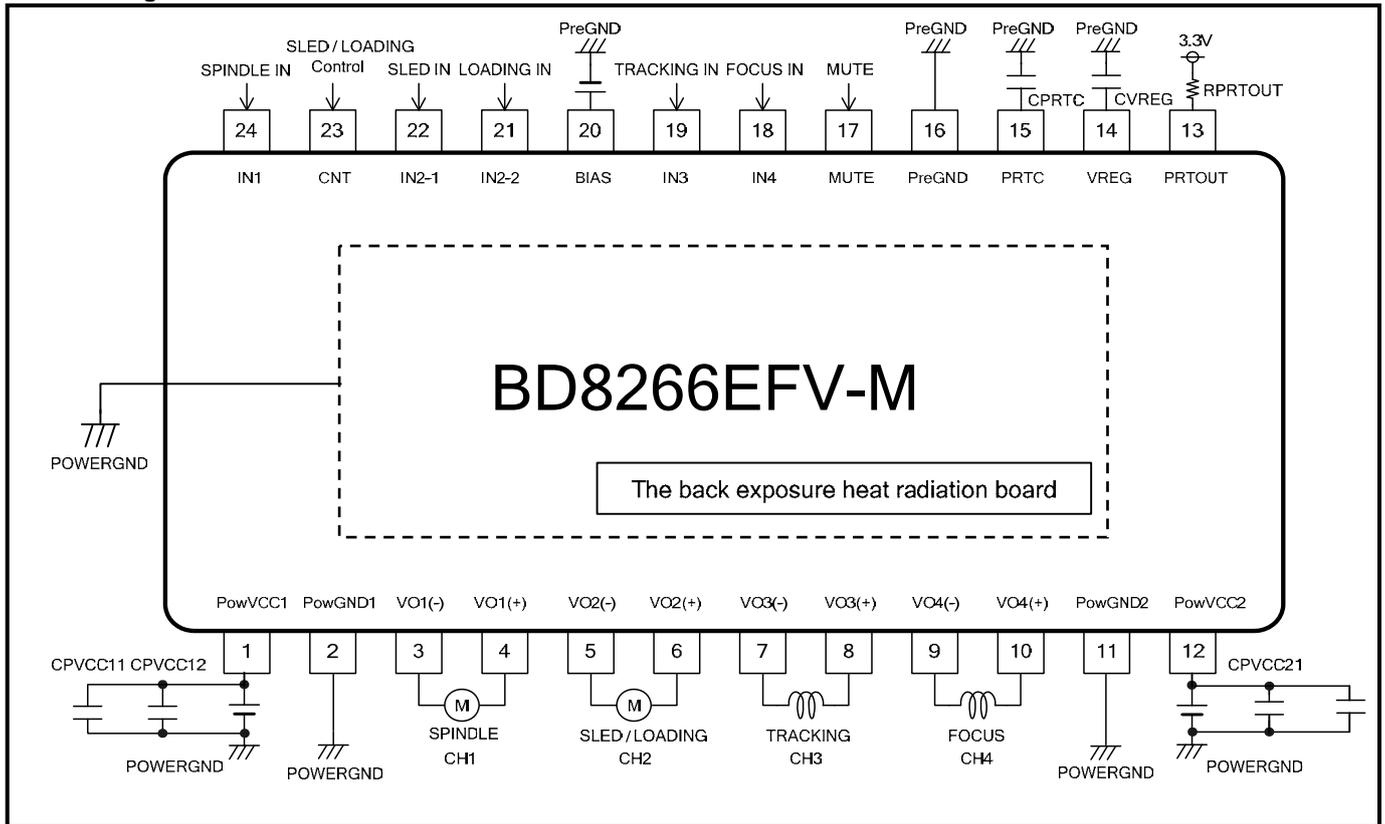
Figure 22. Block Diagram
