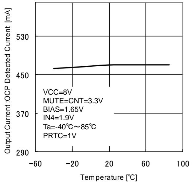
Figure 5. OCP Detected Current
