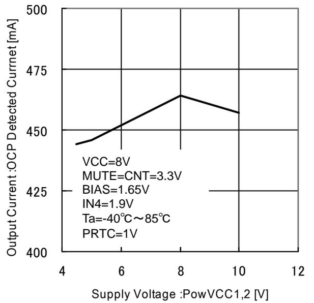
Figure 7. OCP Detected Current
