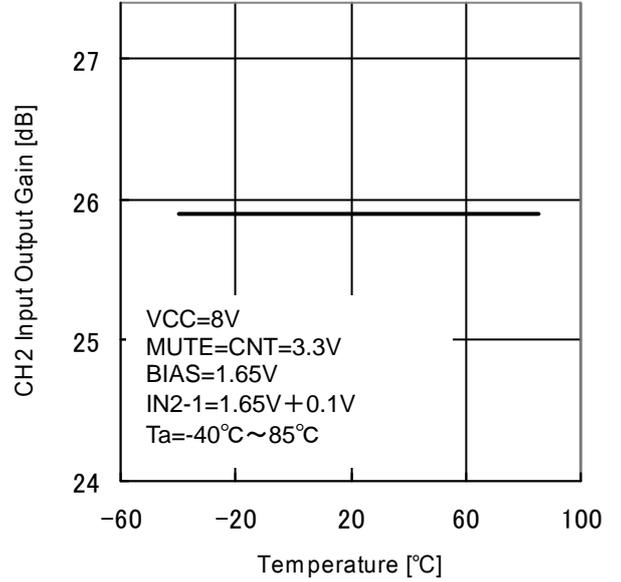
Figure 9. CH2 Closed Loop Gain
