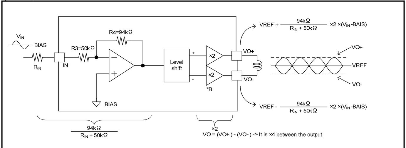
Figure 21. FOCUS, TRACKING Closed Loop Gain calculation
