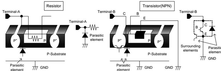
Figure 24. Example of IC Structure
