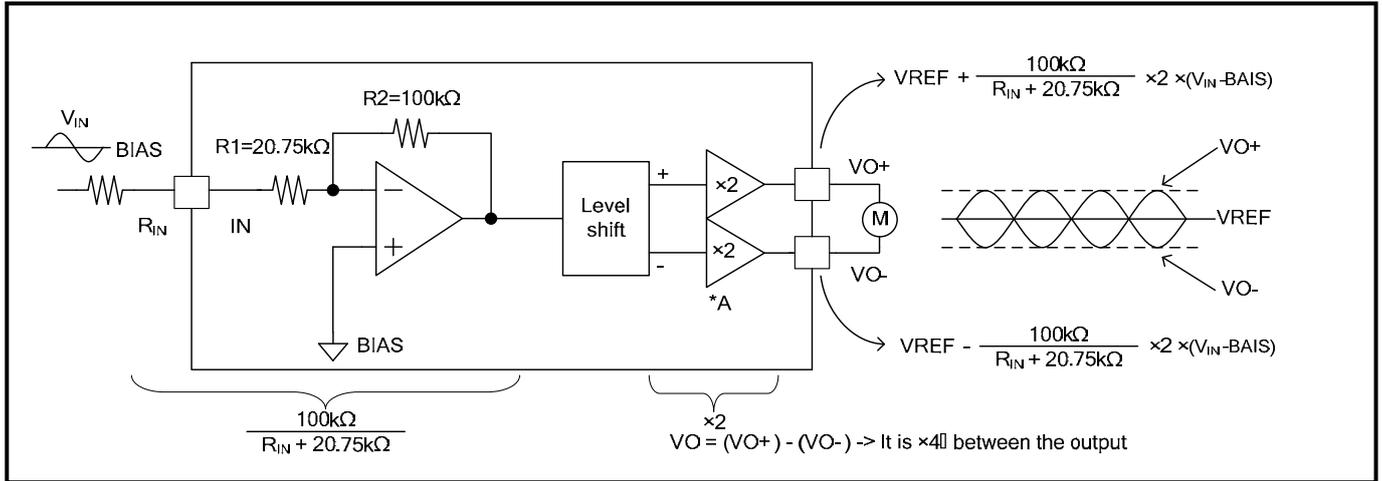
Figure 20. SPINDLE, SLED/LOADING Closed Loop Gain calculation
