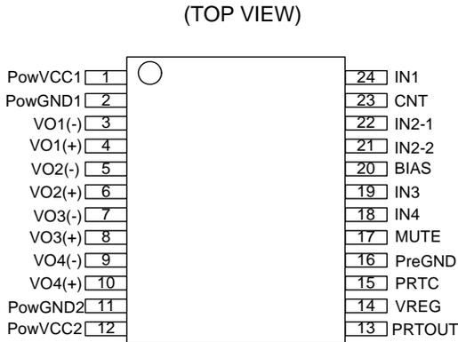
Figure 2. Pin Configuration
