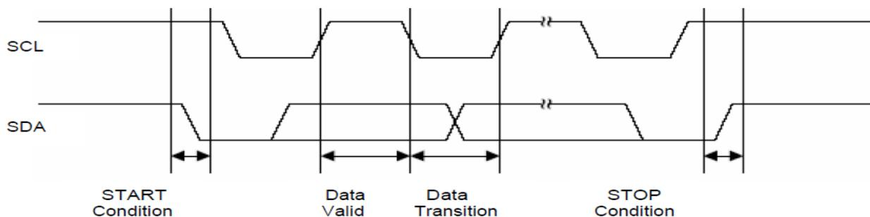
Figure 3: Timing diagram for start and stop conditions
