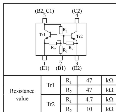
■ Electrical Characteristics  $T_a = 25^\circ\text{C} \pm 3^\circ\text{C}$
