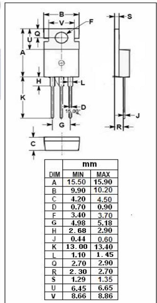
**isc N-Channel MOSFET Transistor****IPP034N03L, IIPP034N03L****ELECTRICAL CHARACTERISTICS** $T_c=25^\circ\text{C}$  unless otherwise specified
