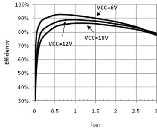
Figure 2.11 Efficiency vs. Output Current ( $V_{OUT} = 5V$ )
