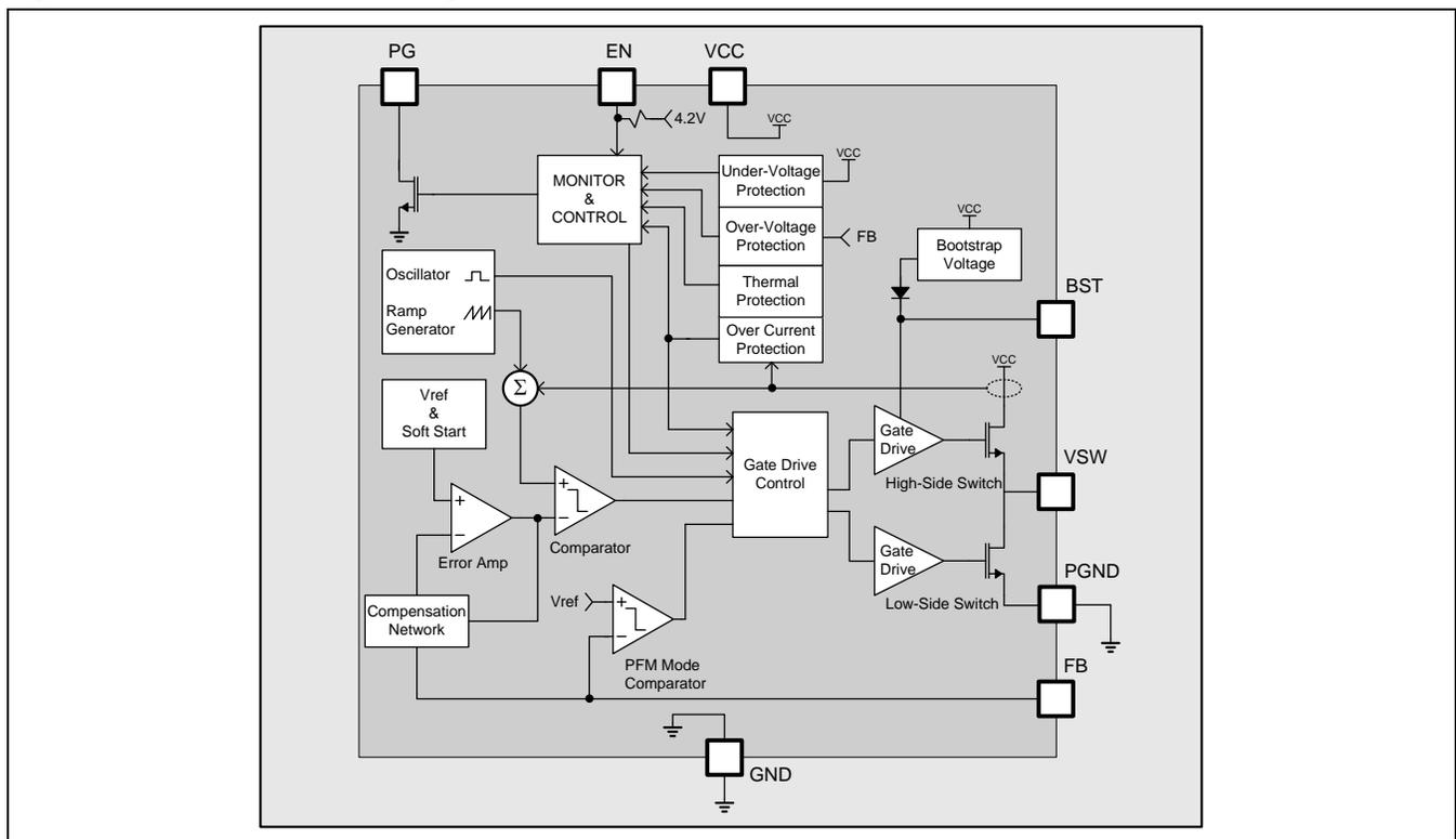
**Figure 3.2 Monitor and Control Logic Functionality**
