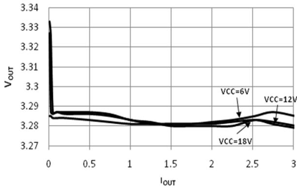
Figure 2.8 Line Regulation ( $I_{out}=1A$ )
