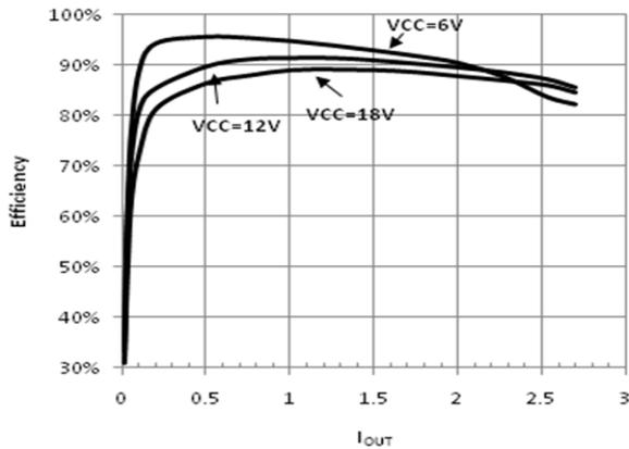
Figure 2.12 Efficiency vs. Input Voltage ( $V_{OUT} = 3.3V$ )
