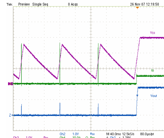
Fig. 9 Shorted Hiccup Condition Recovery
