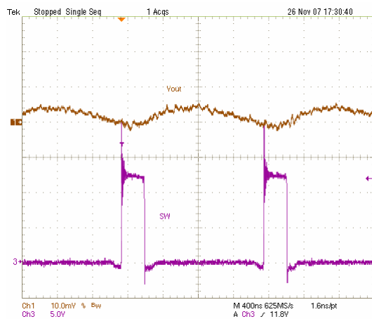
Fig. 6 Output Voltage Ripple at 20A Load
