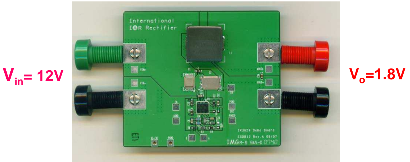
Fig. 1 Connection diagram of the evaluation board for IR3629 (Top view)
