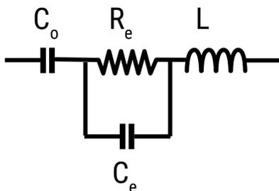
$C_o$  = Aluminum oxide capacitance (surface and thickness of the dielectric)
