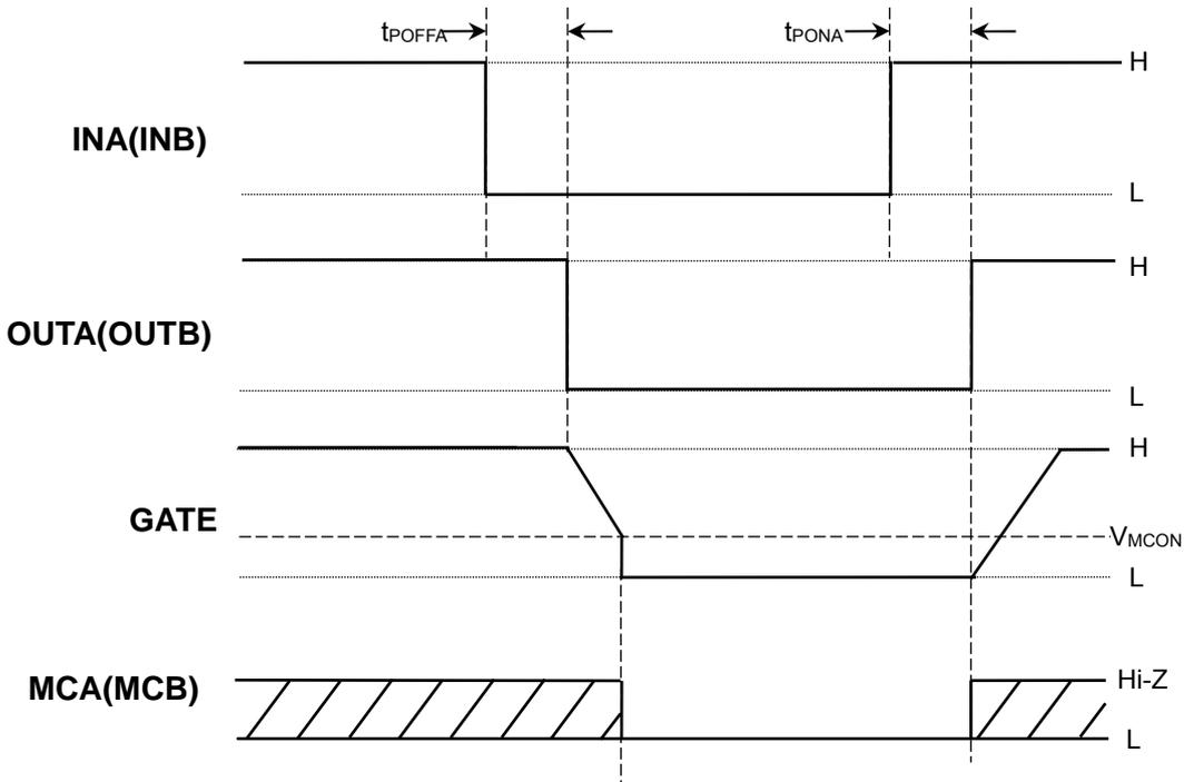
Figure 3. Timing chart of Miller Clamp function
