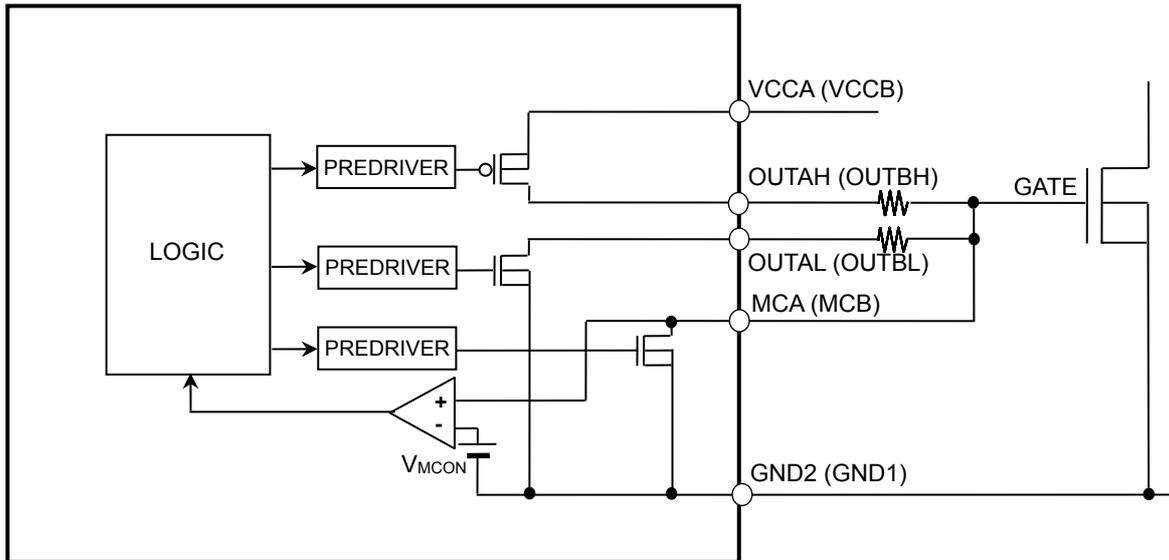
Figure 2. Block diagram of Miller Clamp function.
