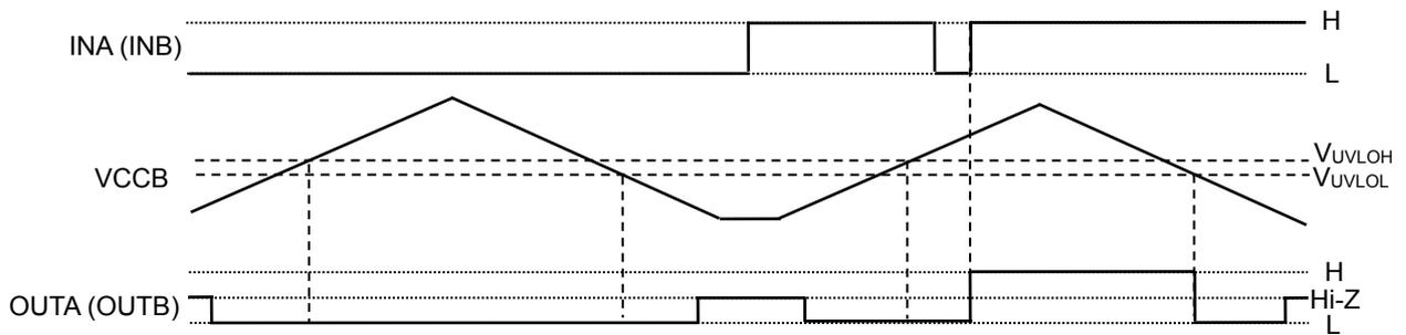
Figure 5. Output-side UVLO Function Operation Timing Chart
