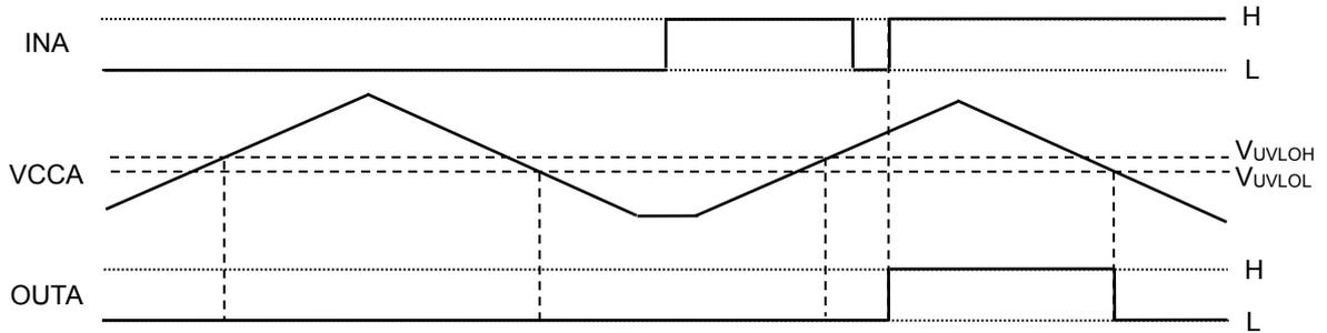
Figure 4. Input-side UVLO Function Operation Timing Chart
