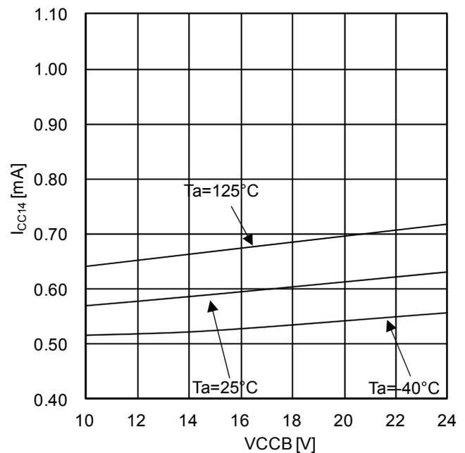
Figure 11. VCCB circuit current 4 (INA=20kHz, Duty=50%)
