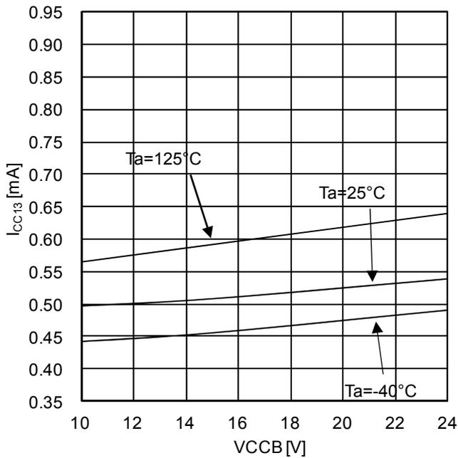
Figure 10. VCCB circuit current 3 (INA=10kHz, Duty=50%)
