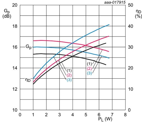
$V_{DS} = 28\text{ V}$ ;  $I_{Dq} = 110\text{ mA}$ ;  $T_{case} = 25\text{ °C}$ ; carrier spacing = 5 MHz; 46 % clipping; PAR = 8.4 dB at 0.01 % probability on CCDF.
