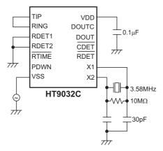
Supply current testing: All, except PDWN and RTIME, unwired pins are left floating.
