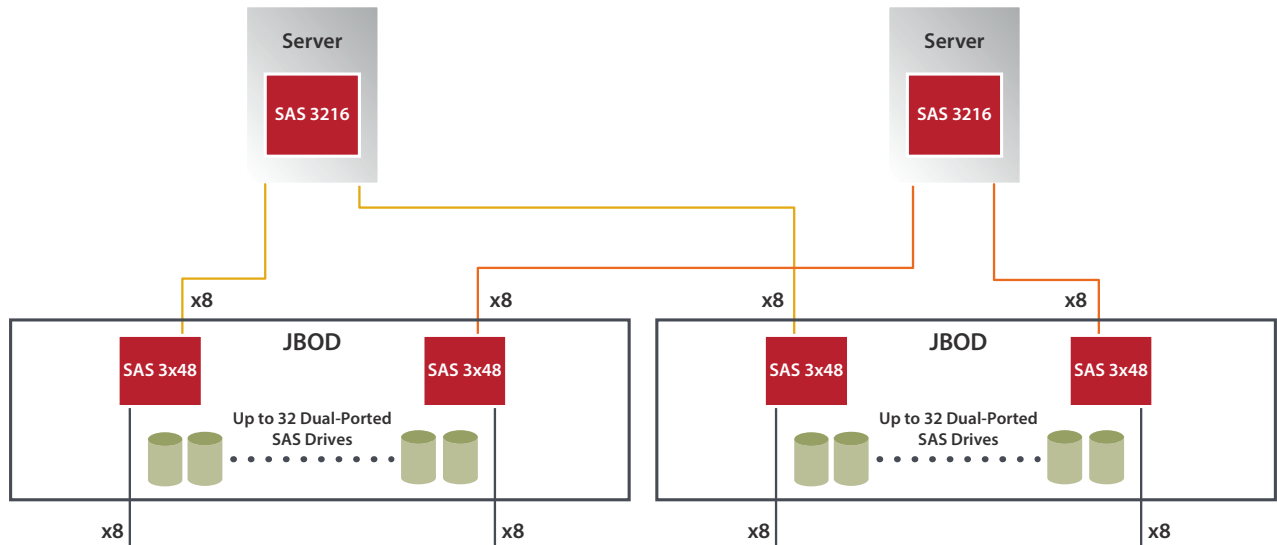
Figure 3: SAS 3216 Topology Diagram
