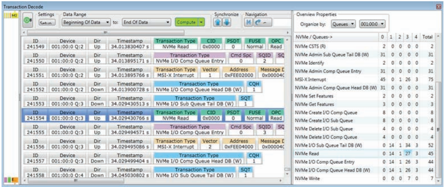
Figure 7. NVMe transaction information provides easy to understand displays of NVMe payloads and PRP messages. The transaction overview of all transactions enables instant access to all messages in the captured trace.
