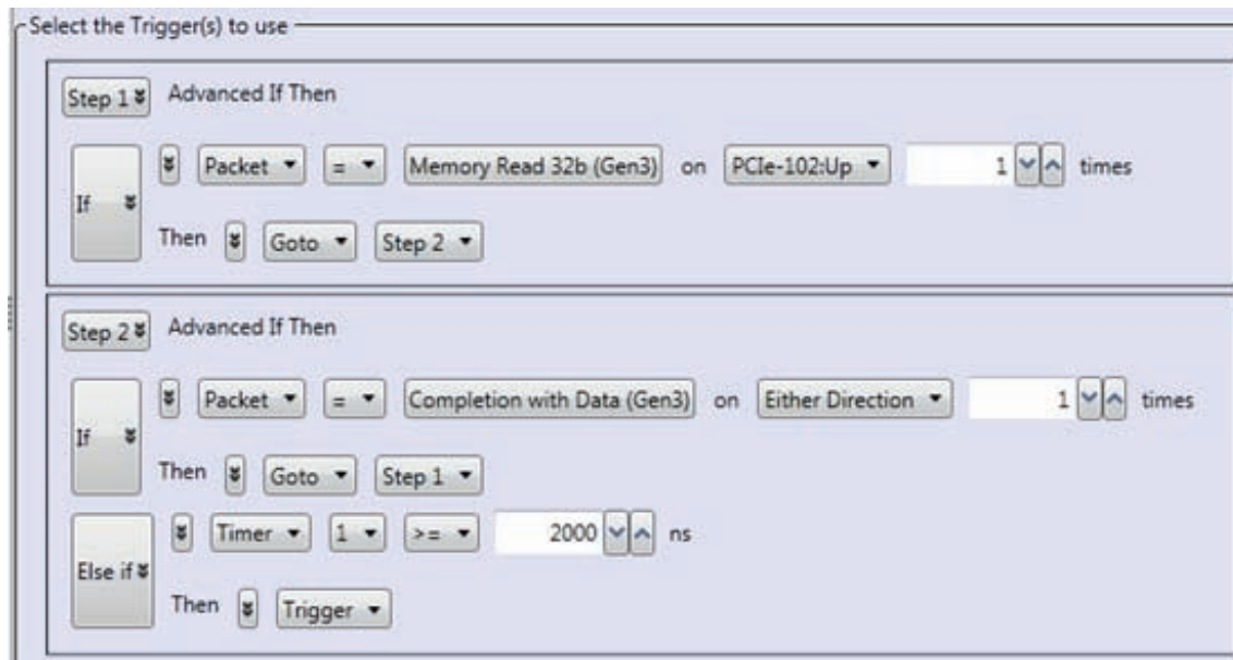
Figure 6. Advanced state-based trigger captures the timeout of a completion packet that takes longer than 2 \mu s.
