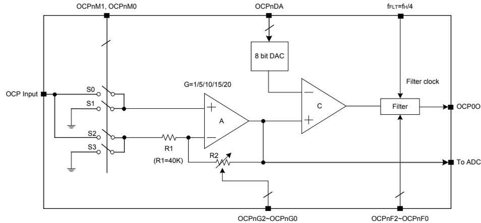
**Over Current Protection Block Diagram (n=0 or 1)**
