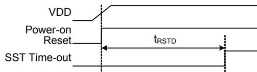
Note:  $t_{RSTD}$  is power-on delay, typical time=16.7ms
