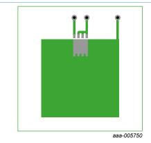
Fig. 5. PCB layout for thermal resistance junction to ambient 1" square pad; FR4 Board; 2oz copper
