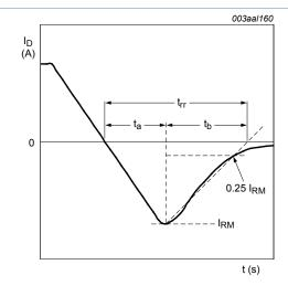
Fig. 16. Reverse recovery timing definition
