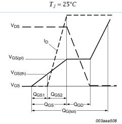
Fig. 12. Gate charge waveform definitions
