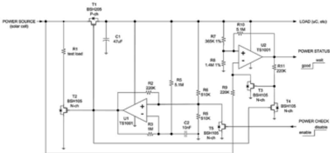
**Figure 3. An Ultra-Low-Power Op-Amp-based Circuit Assesses A Pv Solar-Cell Source**
