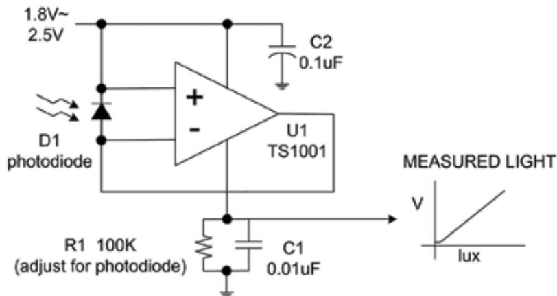
**Figure 2. An Ultra-Low-Power Op Amp Offers Simple, Positive Polarity Output to Support a Zero Bias Condition**
