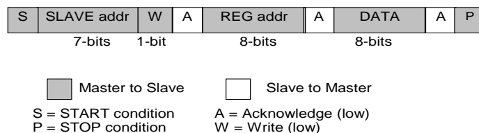
Figure 22: I2C byte write (SDA signal)
