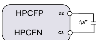
Figure 39: Charge pump flying capacitor
