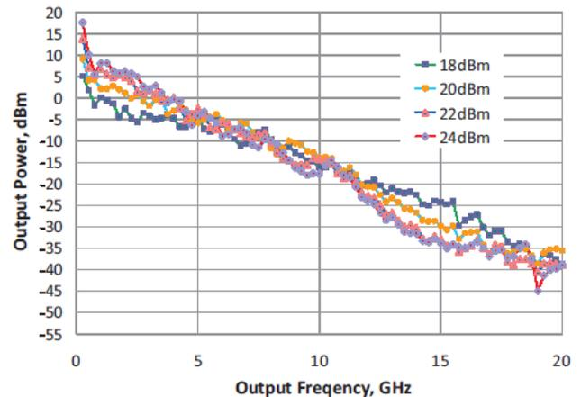
Harmonic Output, 400 MHz Input Frequency
