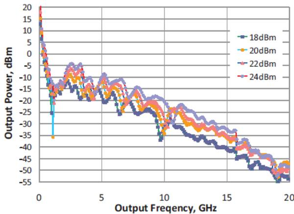
Harmonic Output, 250 MHz Input Frequency
