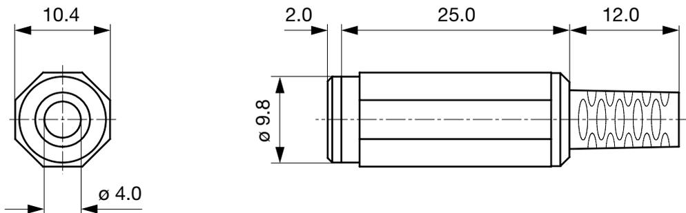
Cable diameter max. 4.0 mm
