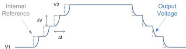
Figure 21. Dynamic Voltage Scaling Effect Timing Diagram
