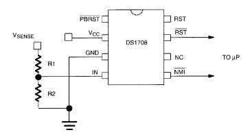
$$V_{SENSE} = \frac{R1 + R2}{R2} \ X \ 1.25 \qquad \qquad V_{MAX} = \frac{V_{SENSE}}{V_{TP}} \ X \ V_{CC}$$
