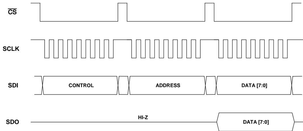
**Figure 17: SPI Read Transaction – 8-bit Mode**
