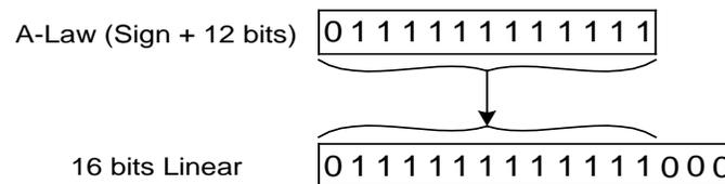
**Figure 24: Mapping of A-law Code to 16-bit Code**
