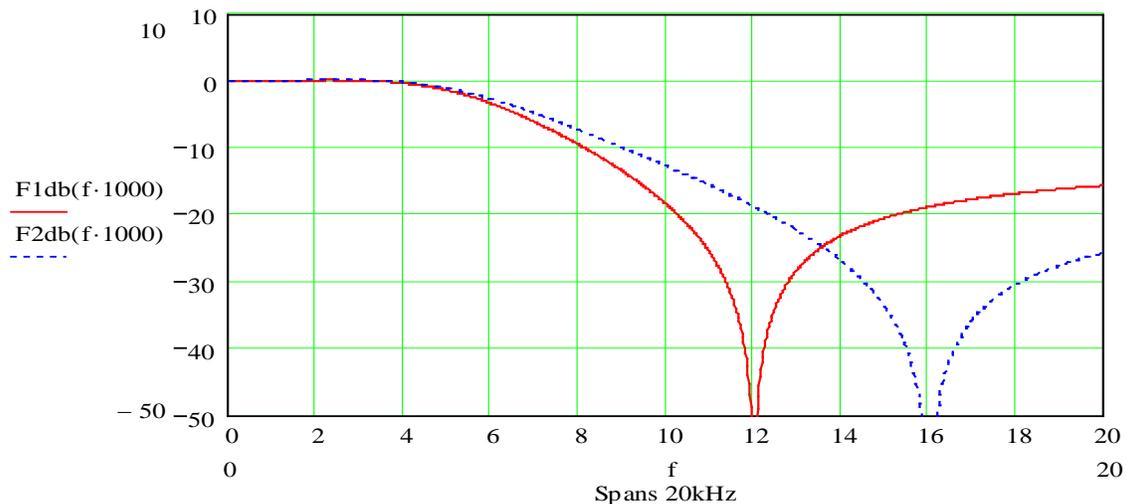
**Figure 37: Magnitude Response of Billing Tone Notch Filter**
