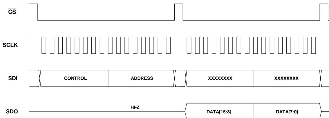
**Figure 19: SPI Read Transaction – 16-bit Mode**
