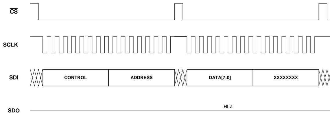
**Figure 18: SPI Write Transaction – 16-bit Mode**
