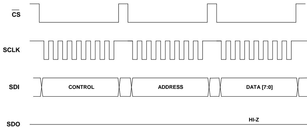
**Figure 16: SPI Write Operation – 8-bit Mode**
