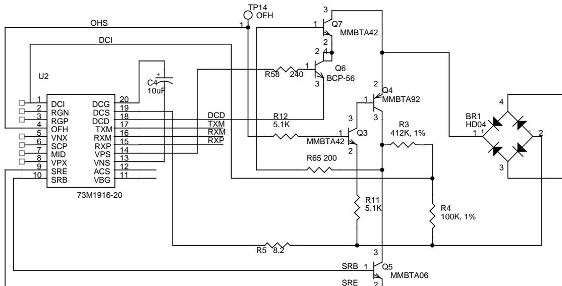
**Figure 32: Line-Side Device AC and DC Circuits**
