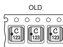
**Packaging** 750/7" reel; 2500/13" reel. Plastic tape: 12 mm wide, 0.32 mm thick, 8 mm pocket spacing, 3.1 mm pocket depth
