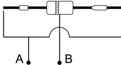
Insulation strength test condition: Apply half sine wave voltage with 10kV wave height between A and B in insulation liquid
