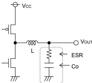
Fig.28 Output capacitor
