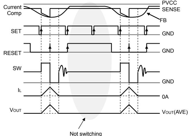
Fig.23 SLLM™ switching timing chart
