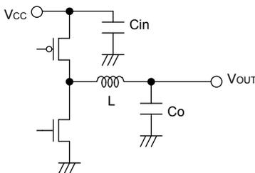
Fig.29 Input capacitor
