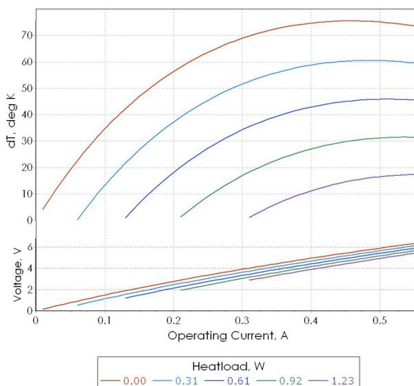
**Note:** Performance data is specified for optimal conditions (TEC hot side is stabilized at ambient temperature). Heatsink thermal resistance is not included into estimations. Use TECCad Software for estimations under different conditions.
